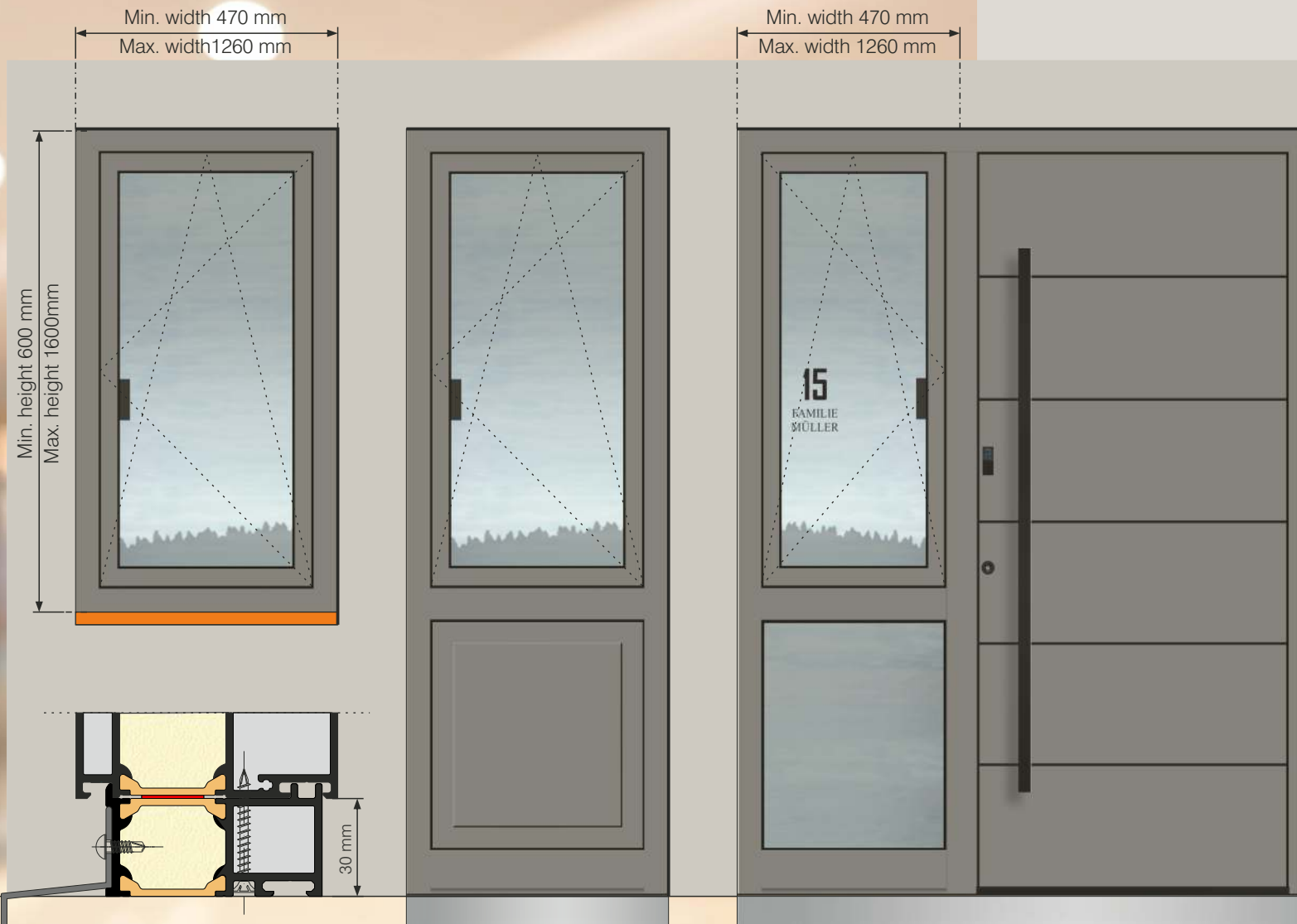
TYP ST 105 sidelight with tilt-and-turn window Cill profile 30mm height
