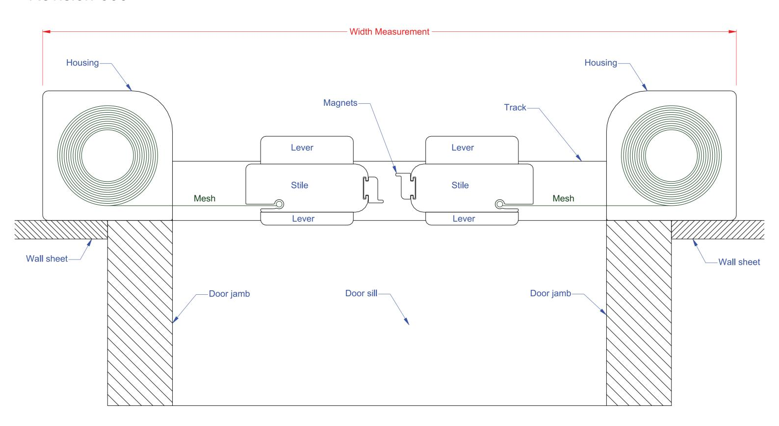
Freedom Screens Zipline PLAN VIEW - INTERNAL CORNER SCALE 1:2 at A3 Revision-006 Mesh Door sill-
